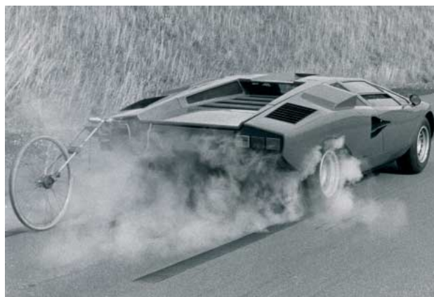
First UK test of the Lamborghinini's acceleration and braking (the wheel at the back measures the true road speed), 1975
